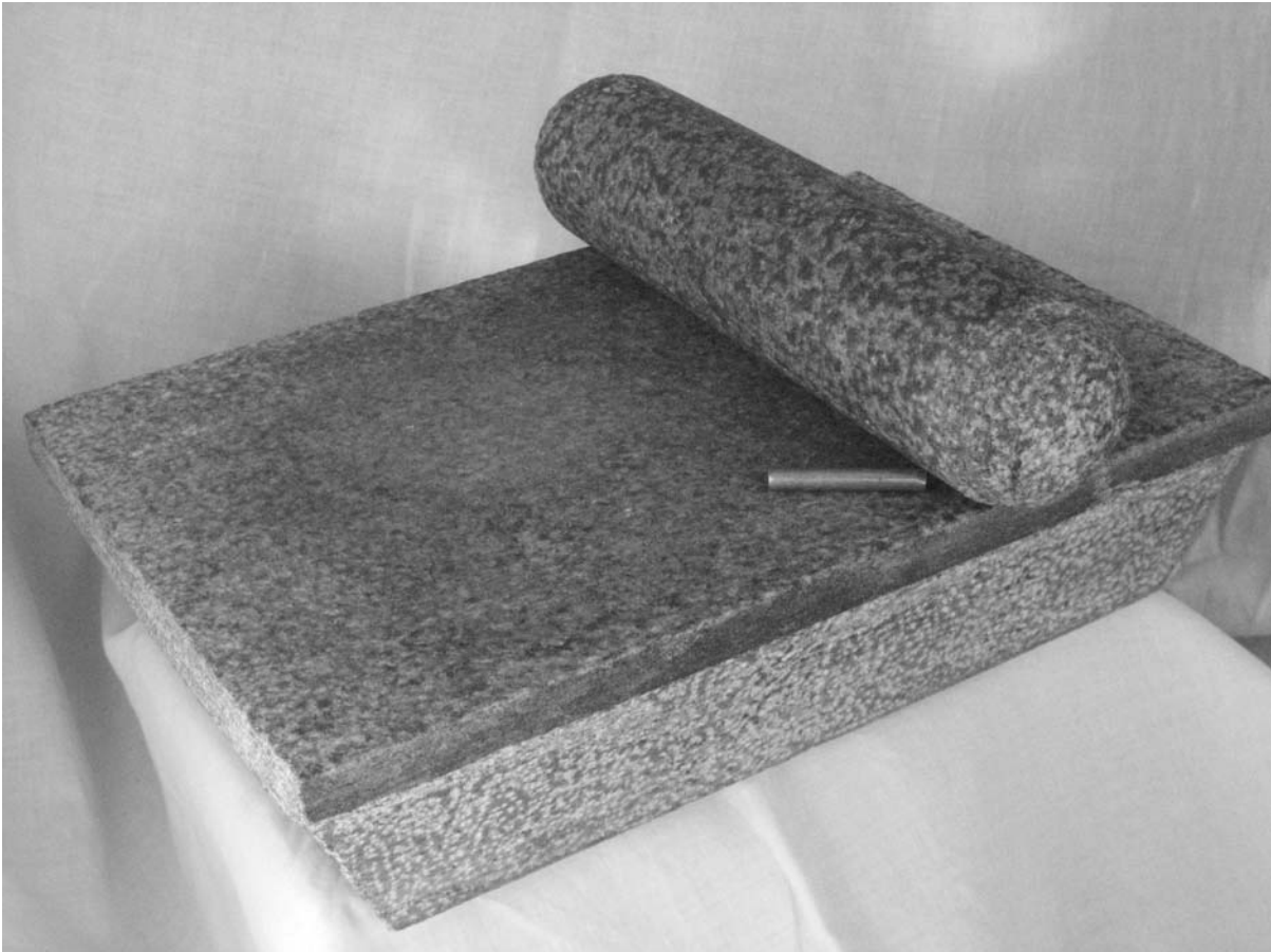
FIG. 1 The modern granite quern used for the grinding experiments. The scale bar is 40 mm.
