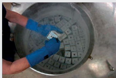
Figure 1. Cryopreservation is used for long-term storage at the National Center for Genetic Resources Preservation in Fort Collins, Colorado. Plant or animal germplasm is placed in a cryotank and submerged in liquid nitrogen or its vapour. © DR DAVID DIERIG.
